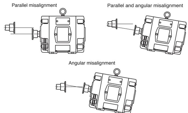
**Figure 3. Types of angular misalignment.**
