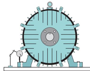
Place a dial indicator to sense upward movement of a motor foot and then loosen the mounting bolt to check for deflection.
